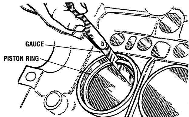
Piston Ring End Gap Limit 0.591 in (1.5mm)
