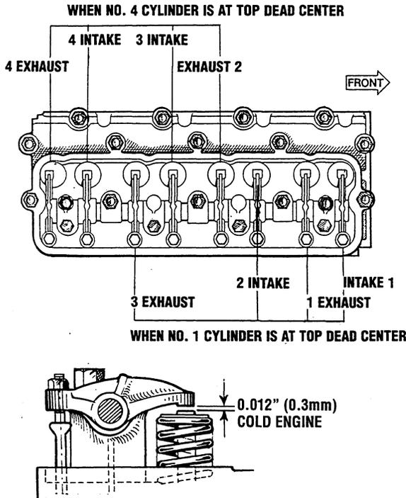
**32. Adjust each valve's clearance** by inserting a 0.012 in (0.03 mm) feeler gauge between the rocker arm and the valve stem.
