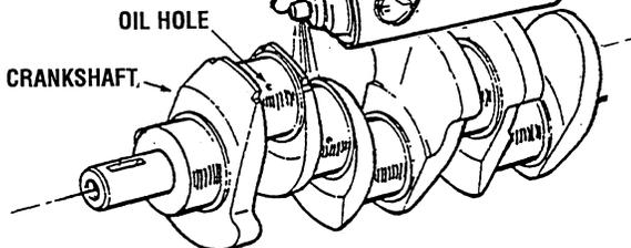
Check for clogging of oil passages and, if clogged, remove with compressed air or a wire.
