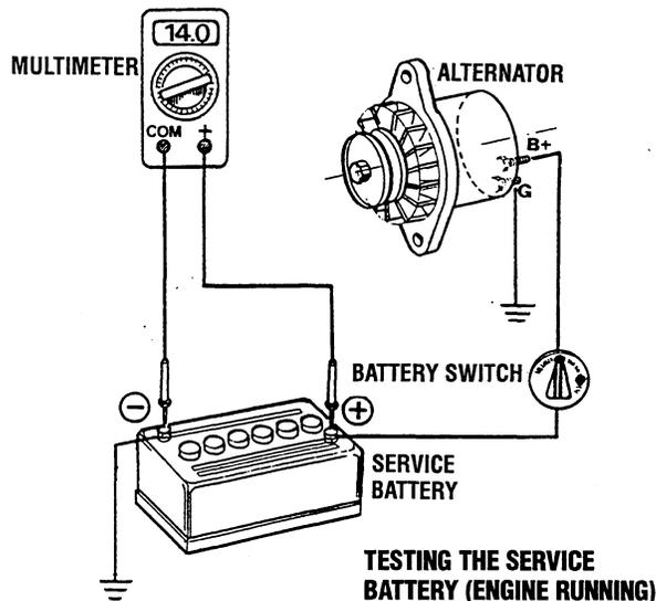
**CAUTION:** When performing tests on the alternator charging circuit do not use a high voltage tester (i.e. Megger). You can damage the alternator diodes.
