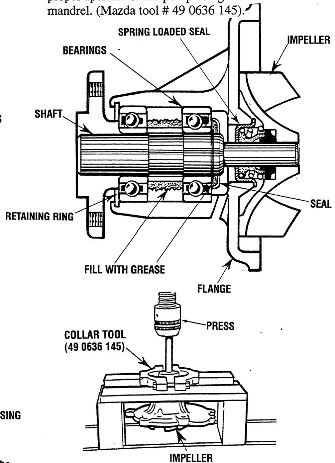
**NOTE:** Do not allow oil or grease to contaminate the surfaces of the ceramic ring or the graphite (small end) of the spring-loaded seal.
