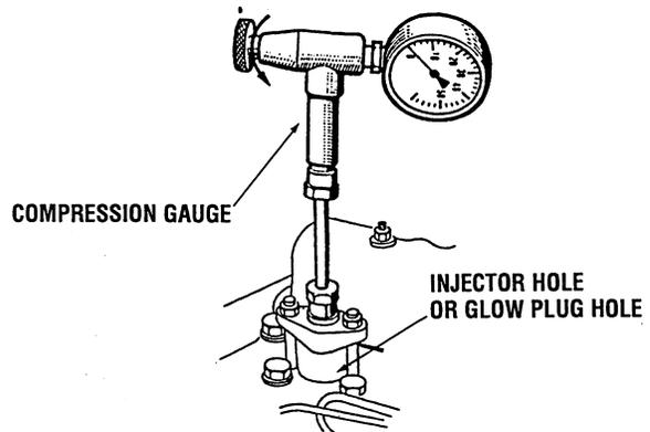
Compression pressure standard 427 psi at 200 rpm (30.0 kg/cm<sup>2</sup>)
