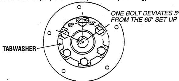
**23. Install the raw water pump.** Mount the raw water pump on its adapter plate and assemble it to the engine. Do not tighten.
