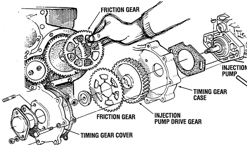
28. Remove the timing gear cover and remove the injection pump washer, injection pump friction gear and the injection pump drive gear.
