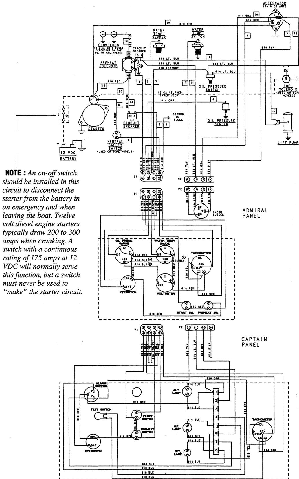
**NOTE :** An on-off switch should be installed in this circuit to disconnect the starter from the battery in an emergency and when leaving the boat. Twelve volt diesel engine starters typically draw 200 to 300 amps when cranking. A switch with a continuous rating of 175 amps at 12 VDC will normally serve this function, but a switch must never be used to "make" the starter circuit.
