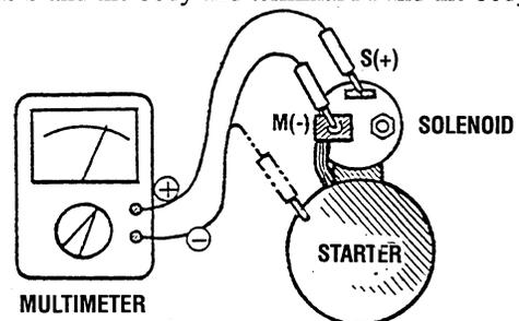
**NOTE:** Disconnect the wire from terminal M.
