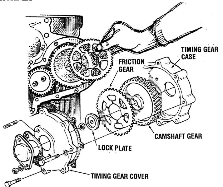
**13. Install the friction gear.**
