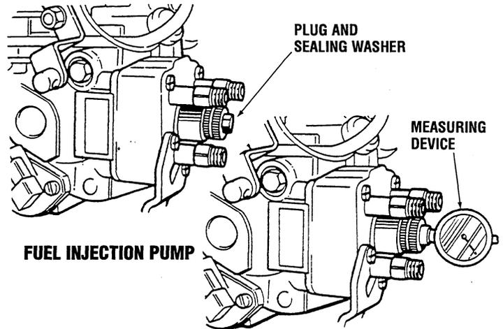
**NOTE:** When setting the dial gauge, confirm that the dial gauge pointer does not deviate from the scale mark of zero by slightly turning the engine crankshaft from left to right.
