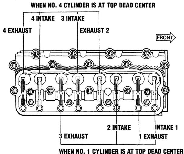
8. Adjust each valve's clearance by inserting a 0.012in (0.03mm) feeler gauge between the rocker arm and the valve stem. Make sure to adjust all valves when the engine is cold.
