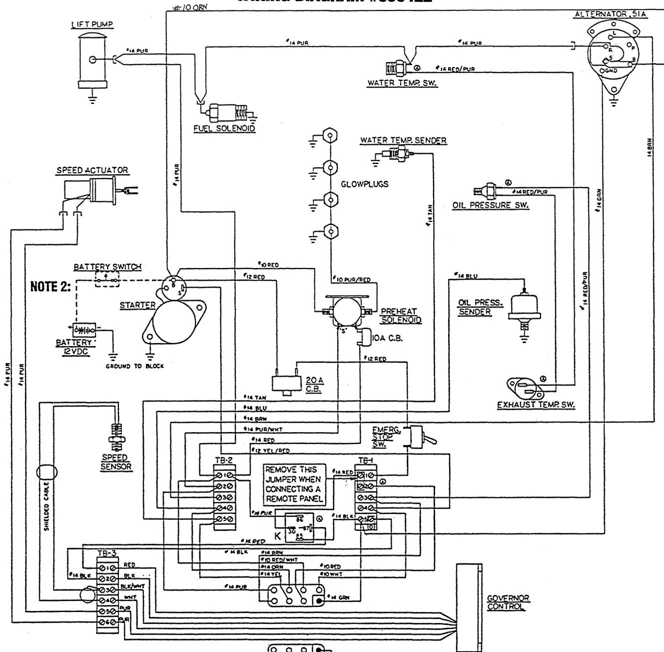
**NOTE 2:** An on-off switch should be installed in this circuit to disconnect the starter from the battery in an emergency and when leaving the boat. Twelve volt diesel engine starters typically draw 200 to 300 amps when cranking. A switch with a continuous rating of 175 amps at 12 VDC will normally serve this function, but a switch must never be used to "make" the starter circuit.
