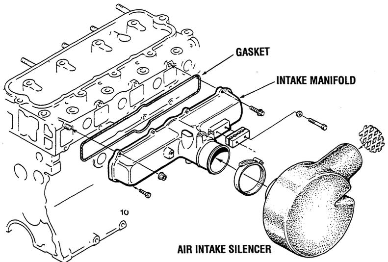
11. Remove the air intake silencer and the intake manifold.
