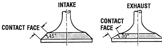
e. Check if the valve seat contact face contacts the center position of the valve contact face. If the contact position is not centered, recut and surface the valve seat and valve.
