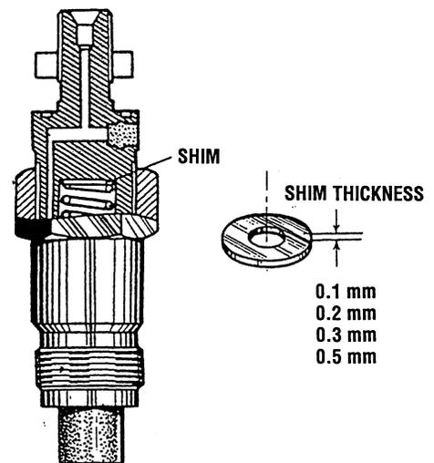
When replacing the shim, grip the retaining nut in a vise and remove the body with a wrench. Tighten the retaining nut to the specified torque.
