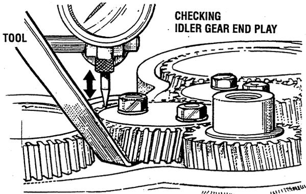
**NOTE:** Measure the end play after tightening the idler gear attaching nuts to the specified torque value.
