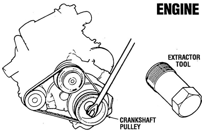
27. Remove the crankshaft pulley bolt with the aid of a 38 mm socket and draw the pulley off the front crankshaft.
