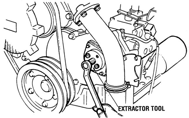
**NOTE:** If an extractor is not available, replace the nut on the injection pump shaft loosely and with a nylon drift and hammer gently tap the injection pump shaft to dislodge it from the keyed drive gear.
