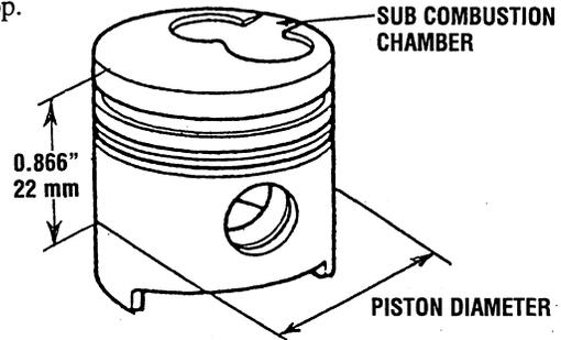
Standard Piston Diameter 3.7381 - 3.7399 in (94.967 - 94.993mm)
