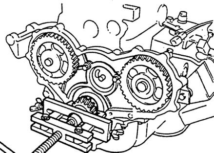
REMOVING THE CRANKSHAFT GEAR
