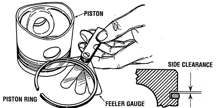
Side Clearance Limit 0.012 in (0.30mm)
