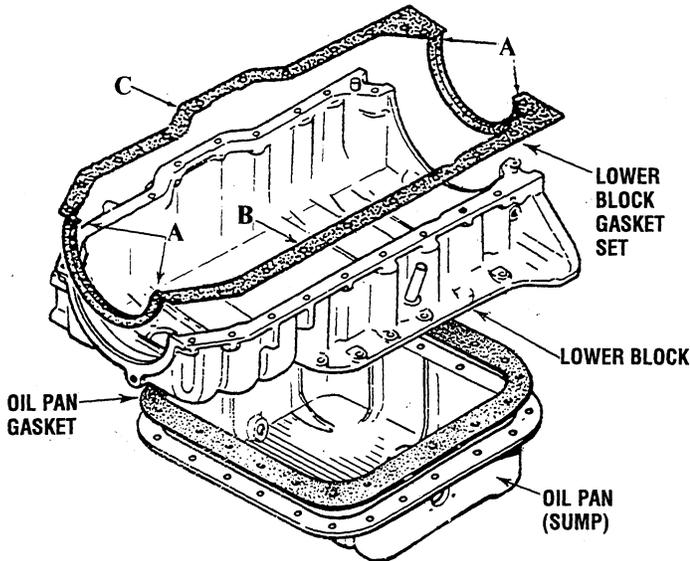
**19. Assemble the new gasket set (lower block).**
