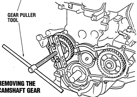
REMOVING THE CAMSHAFT GEAR
