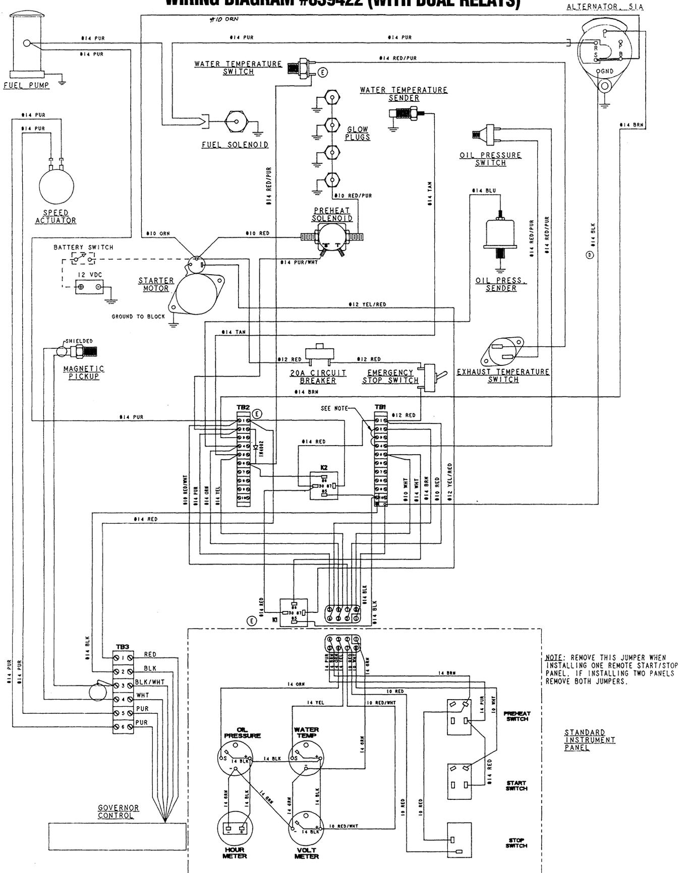
NOTE: REMOVE THIS JUMPER WHEN INSTALLING ONE REMOTE START/STOP PANEL. IF INSTALLING TWO PANELS REMOVE BOTH JUMPERS.
