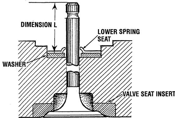
d. Check for contact between the valve and valve seat by applying a thin coat of Prussian Blue (or Redlead) on the valve seat contact face, then insert the valve into the valve guide and press fit the valve on the valve seat.
