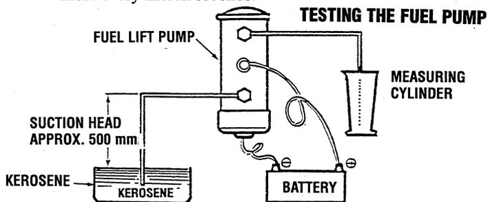
**NOTE:** Later model WESTERBEKE engines and generators use a solid state fuel lift pump that requires no maintenance. The above tests can be performed on these models.
