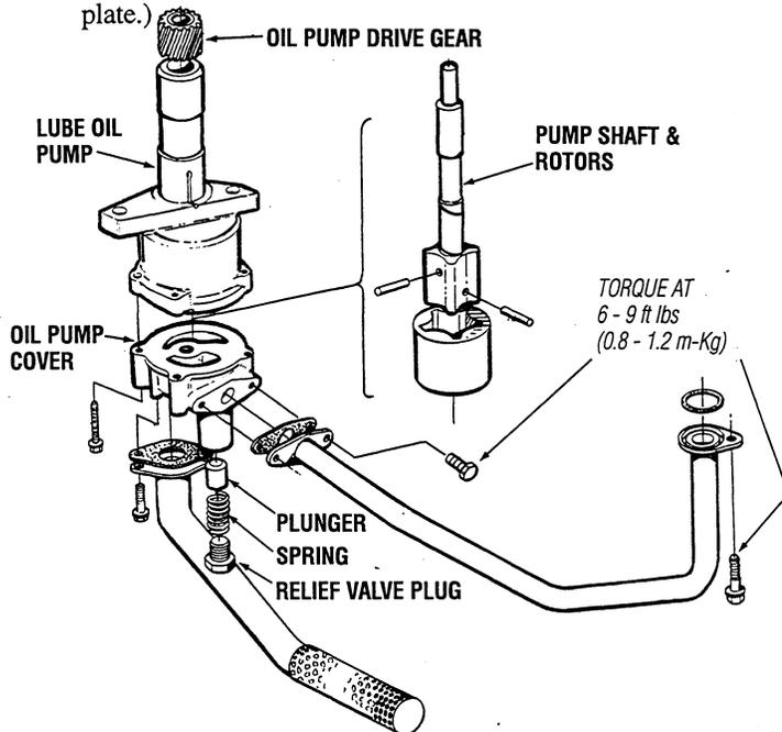
2. **Inspect the clearance between the pump body and the shaft.** Measure the clearance with a dial gauge and magnet base. When the clearance exceeds the limit, replace the pump drive shaft inner rotor, pump body and drive gear.
