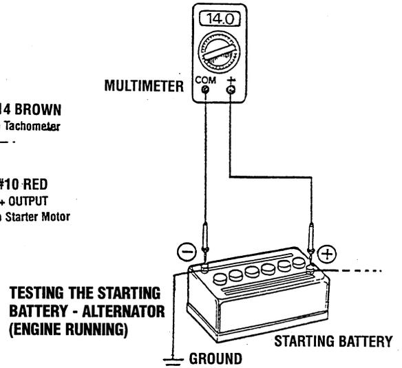
3. If the starting battery voltage remains around 12 volts after the engine is started and run for a few minutes, a problem exists with the alternator or the charging circuit.
